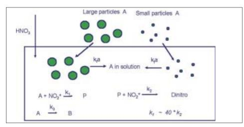
Fig. 11. Process scheme for nitration example
