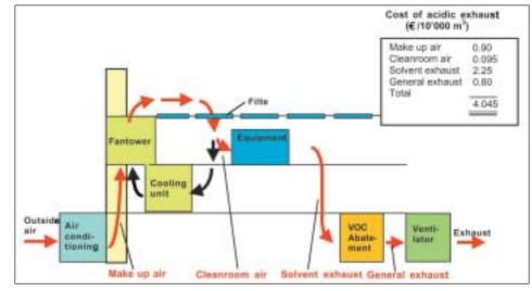
Fig. 2. Calculation of operational costs for the treatment of solvent exhaust from a process equipment located in a cleanroom environment. The costs are based on local prices for electricity, water and wastewater at yearly average climatic conditions in Central Europe.
