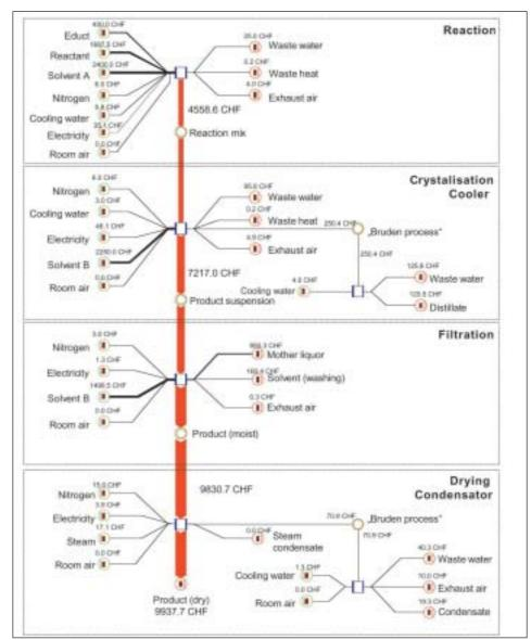
Fig. 3. Mass, energy, and cost flow analysis of a chemical synthesis. The illustration shows cost flows only. All supply and disposal cost flows for each process step are allocated to the final product costs (vertical arrow). The thickness of the single cost flow lines is proportional to the overall costs.
