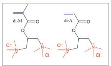
Fig. 1. Chemical structures of the cationic double-charged monomers di-M and di-A. charged flexible PEL, and to synthesize and test novel homo- and copolymers.
