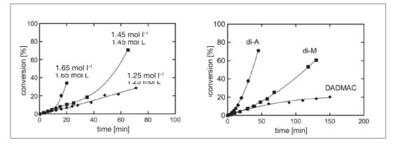
Fig. 2. Auto-acceleration. Left: for different di-M concentrations, right: at 1.25 mol ×  $F^1$  for different monomers. For the less charged diallyldimethylammonium chloride (DADMAC), autoacceleration was even not observed at 4 mol ×  $F^1$ .
