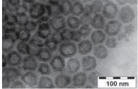
Figure 1. TEM image of CuS hollow spheres.
