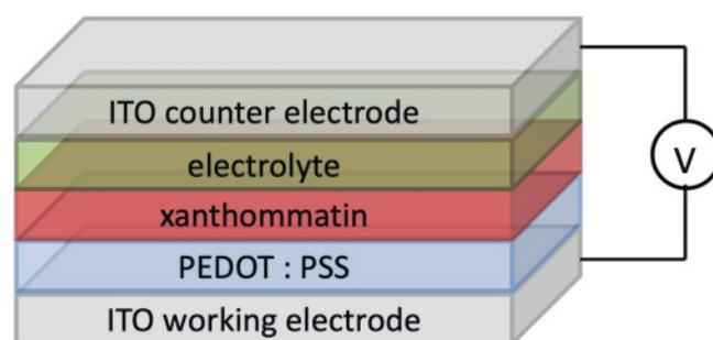
Fig. 3. Device architecture for the xanthommatin-based ECDs reported by Deravi.<sup>[6]</sup>
